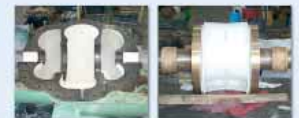
Repair the worn and corroded shaft using Loctite® 3478 Superior Metal. After it's cured, machine it to complete the repair. Coat all parts with Loctite® Nordbak® 7228 Brushable Ceramic White (certified for use in contact with drinking water).
